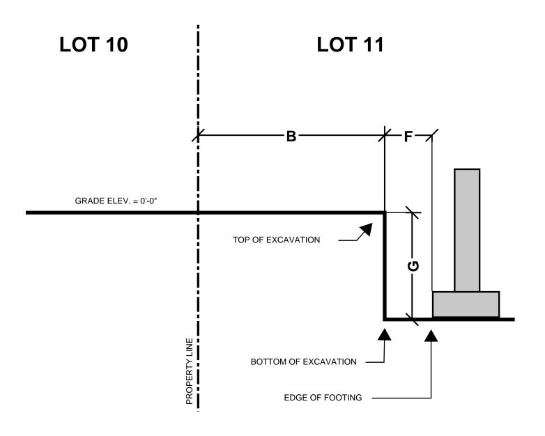
VERTICAL CUTS 4'-0" OR LESS ARE PERMITTED IF THE DISTANCE FROM THE PROPERTY LINE TO THE TOP EDGE OF THE EXCAVATION CUT IS GREATER THAN OR EQUAL TO THE DEPTH OF EXCAVATION.
