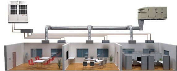
Variable Refrigerant Flow (VRF) Schematic
