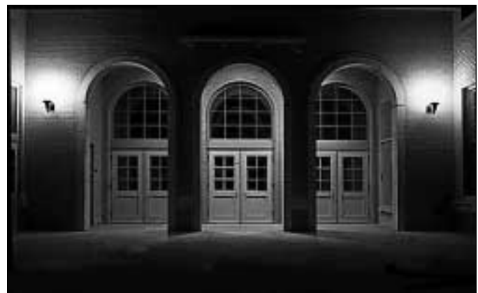
Glare is greatly reduced when the lamp source is hidden from view. Photo by Roger Whitacre.
