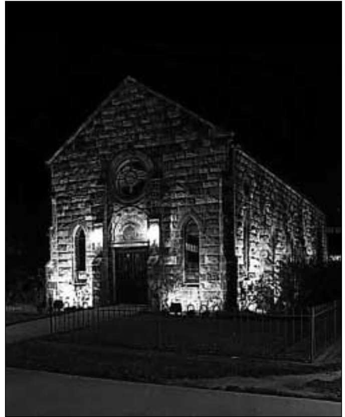
High intensity discharge (HID) lamps are intense sources that require careful placement and shielding from view. HIDs are common in exterior use for floodlighting and street lighting. Photo by Roger Whitacre.
