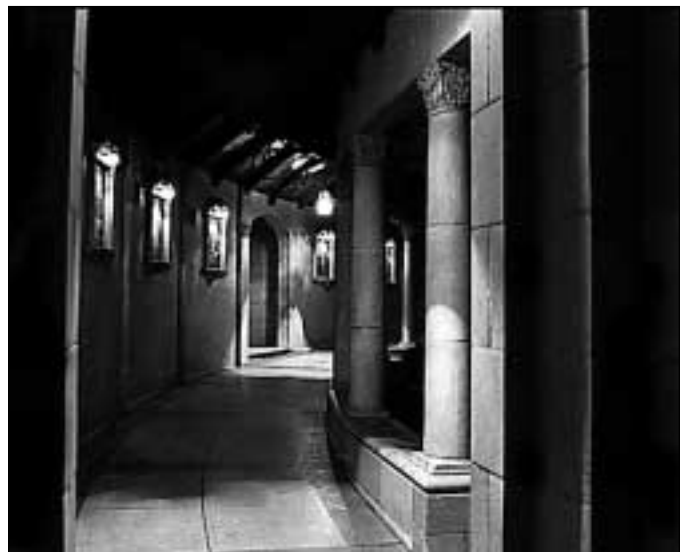
A light-colored background behind lanterns or globes reduces source glare. The glare of globes against a black night background makes seeing difficult. Photo by Roger Whitacre.
