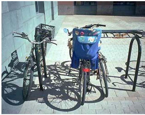
Installing inverted U type racks 30" on center allows for all bicyclists to use them, including parents carrying their children in child seats."
